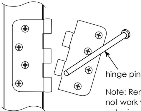
Note: Removal of hinge pin will not work with spring or fixed pin outswing application.
